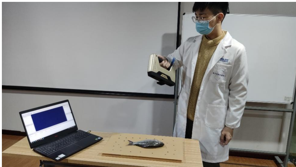
Supplementary Figure S1. Data acquisition via non-contact fish scanning using GScan. Mark points were labeled on a yellow board as background. Point cloud was transferred directly to 3DPhenoFish for analysis.
